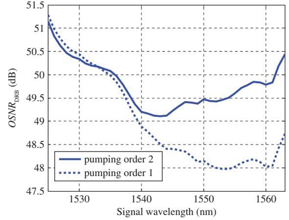
Fig. 5.  $OSNR_{DRB}$  spectrum in the TDM-pumped RAs with four pumps with different pumping orders.
