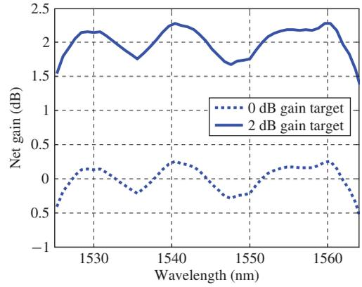
Fig. 1. Net gain spectrum of the optimized RA with the SMF28e fiber.
