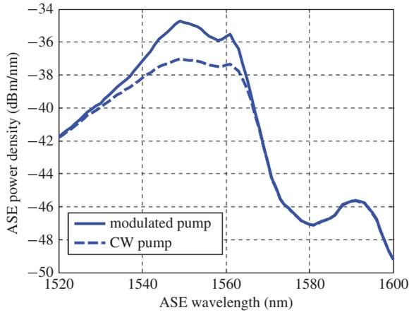
Fig. 4. ASE power spectral densities at the output of the amplifiers with a TDM pump and a CW pump.
