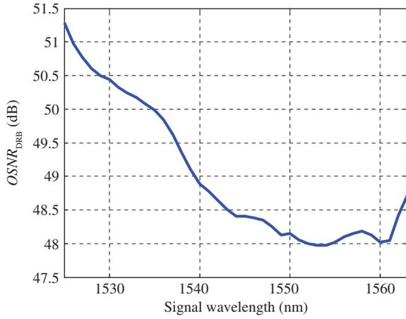
Fig. 3.  $OSNR_{DRB}$  spectrum in a TDM-pumped RA with four pumps. The pump modulation frequency is 8 MHz.
