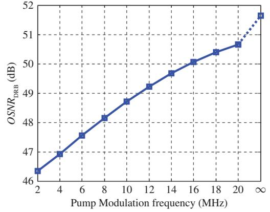
Fig. 2. Impact of the modulation frequency on  $OSNR_{DRB}$  in a TDM-pumped RA with four pumps.
