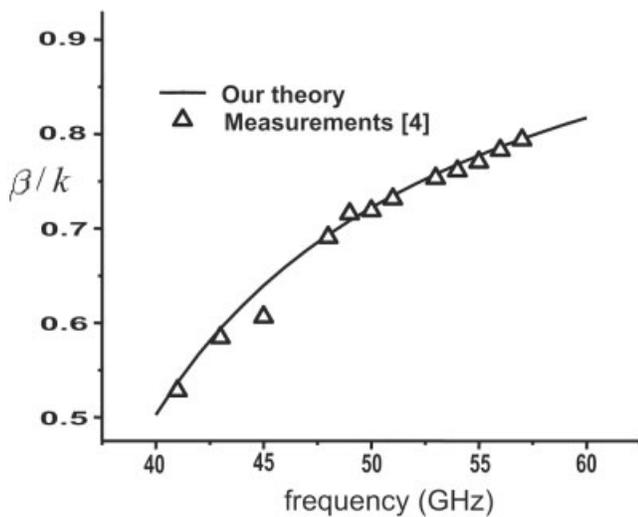
**Figure 2** Behavior of  $\beta$  versus frequency.  $a_1 = 1$  mm,  $a_2 = 1.4$  mm,  $b = 2.3$  mm,  $c = 2.4$  mm,  $d = 3.12$  mm
