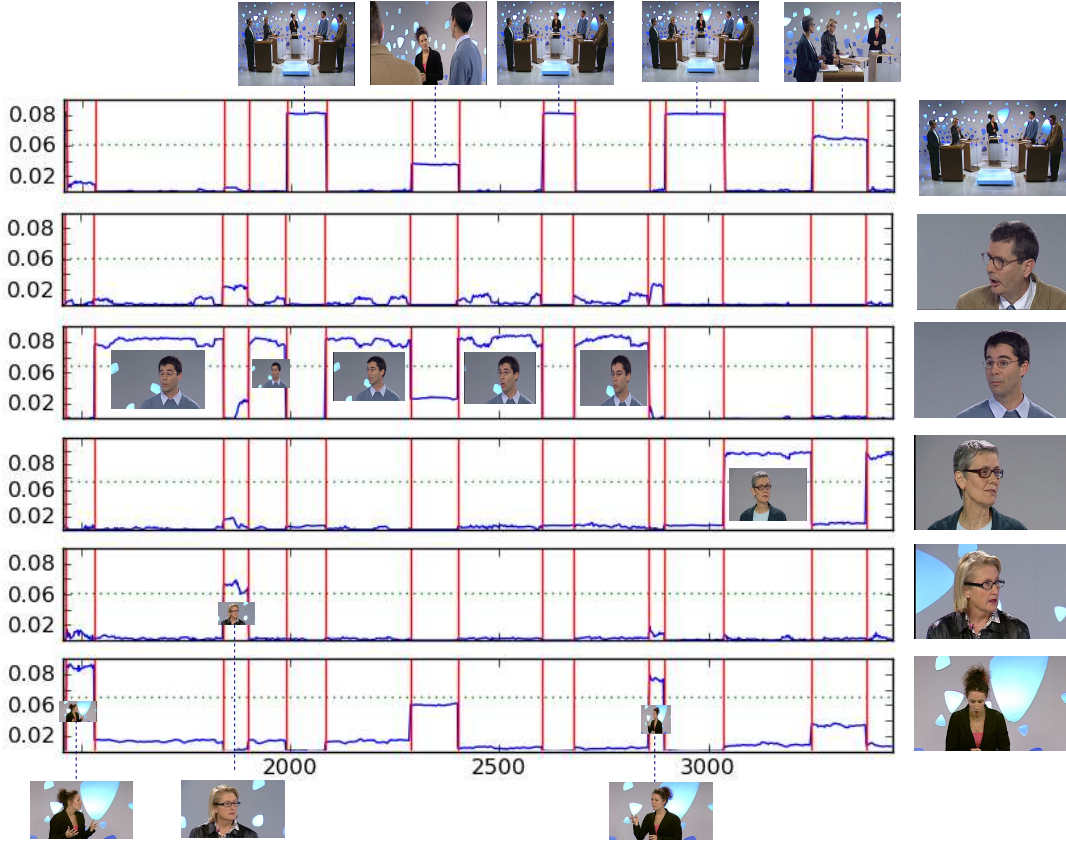
Fig. 4. KL-NMF activations i.e. H coefficients on a short excerpt of the development video with \beta = 0 . Each subplot represents the temporal sequence of activations for one w_k component, 1 \leq k \leq K = N_{sp} + 1 . For each component, the image on the right corresponds to the frame where the activation value is maximum, which is supposed to be a good representative of the content modeled by the corresponding w_k component. Red vertical lines are groundtruth shot boundaries and the other images inside the plot or around it are key frames of the time-corresponding shots. Green dotted horizontal lines are decision thresholds. It can be seen that NMF has succeeded in extracting the relevant components and related activations. Note that the 2nd component is not activated here as the corresponding person does not appear in any personal shot of this part of the video.
