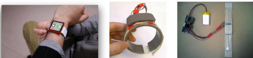
Figure 12: Mockup, First and final prototypes (with Arduino Fio, BlueTooth shield and battery)
