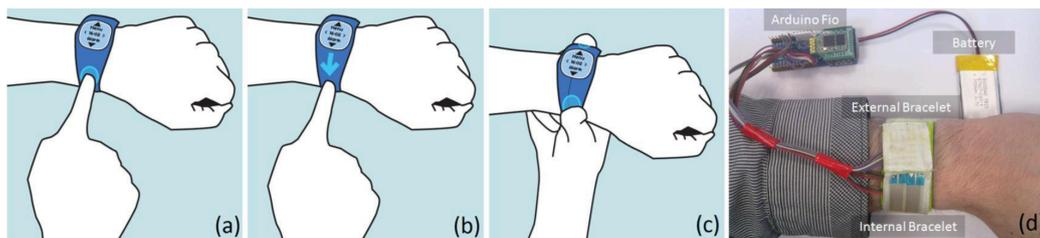
Figure 11: WatchIt: (a) pointing, (b) sliding, (c) with two fingers, (d) experimental prototype
