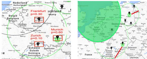
(e) When disks are collapsed around geolocated replicas, disks may no longer overlap, and other enumeration/geolocation iteration takes place
