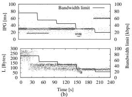
Fig. 3. Active testbed measurement: Skype inter-packet-gap and message size for (a) increasing packet loss rates and (b) decreasing bottleneck bandwidth.
