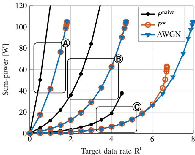
Fig. 1. Sum-power vs. target data rate  $R_k^t = R^t$  with  $G_{\text{amp}} \in \{-10, 0, +10\}$  dB (A, B and C respectively).
