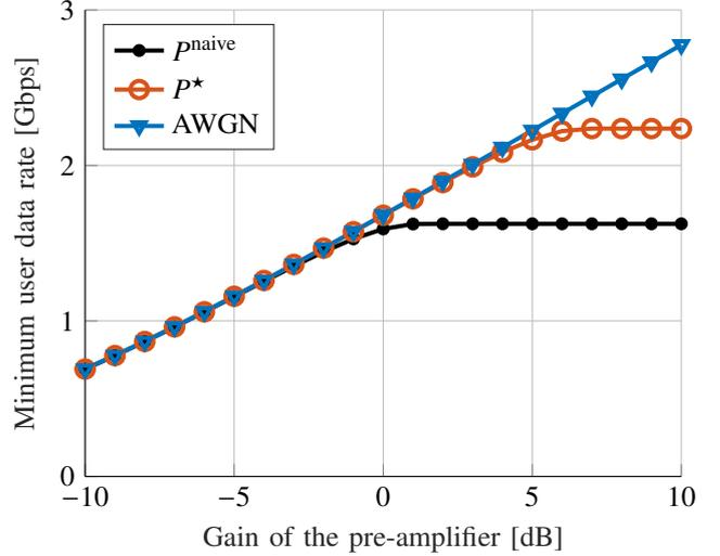
Fig. 2. Minimum of user data rate vs. pre-amplifier gain  $G_{\text{amp}}$ .
