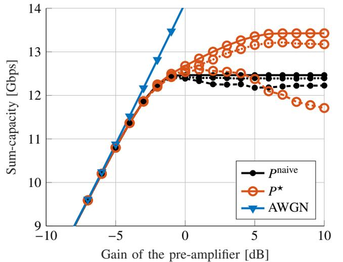
Fig. 3. Sum-capacity vs. pre-amplifier gain  $G_{\text{amp}}$  with  $\epsilon \in \{30, 50\}\%$  (in dotted and dashed line respectively). The solid line is the case of perfect channel gain estimation.
