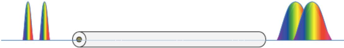
Figure 1.12: Inter-symbol interference due to chromatic dispersion
