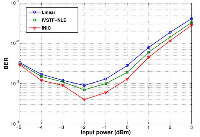
Fig. 5: BER vs. input power for 4-band Dual-Pol-16QAM OFDM
