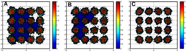
Fig. 3: Constellations: (A) linear equalization; (B) IVSTF-NLE; (C) Proposed INIC
