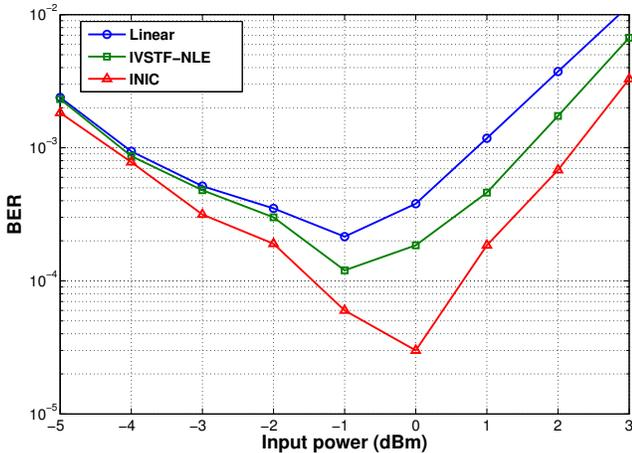
Fig. 4: BER vs. input power for 4-band Single-Pol-16QAM OFDM
