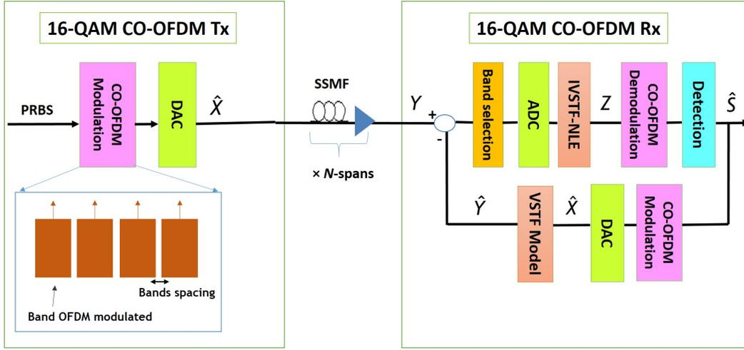
Fig. 1: Transmission diagram
