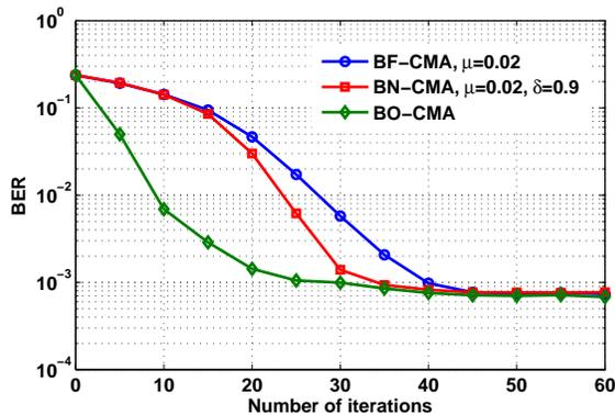
Fig. 1. BER vs. #iterations for block approaches
