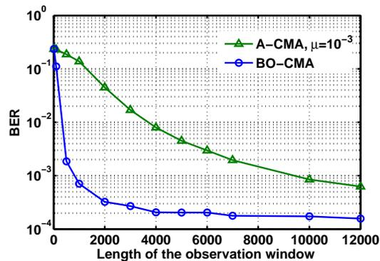
Fig. 2. BER vs. #iterations for adaptive approaches
