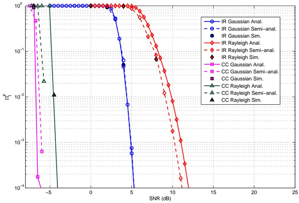
Fig. 7. PER at IP layer for IBS with  $N = 3$ , for CC-HARQ ( $C = 9$ ) and IR-HARQ ( $C = 12$ ).
