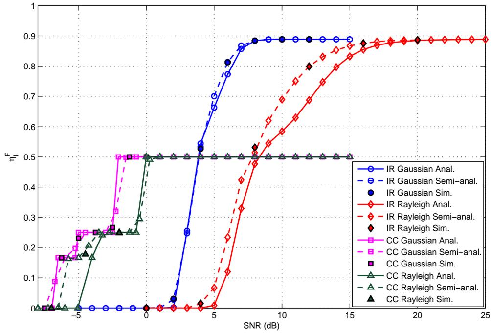
Fig. 4. Efficiency at IP layer for FBS with  $N = 3$ , for CC-HARQ ( $P_{max} = 3$ ) and IR-HARQ ( $P_{max} = 4$ ).
