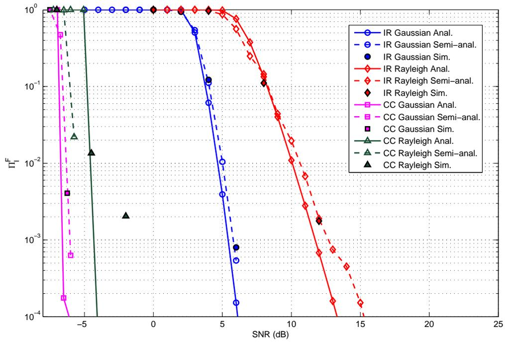
Fig. 8. PER at IP layer for FBS with  $N = 3$ , for CC-HARQ ( $P_{\max} = 3$ ) and IR-HARQ ( $P_{\max} = 4$ ).
