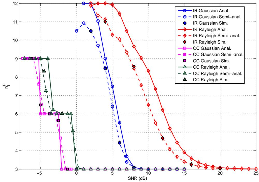
Fig. 6. Delay at IP layer for FBS with  $N = 3$ , for CC-HARQ ( $P_{\max} = 3$ ) and IR-HARQ ( $P_{\max} = 4$ ).
