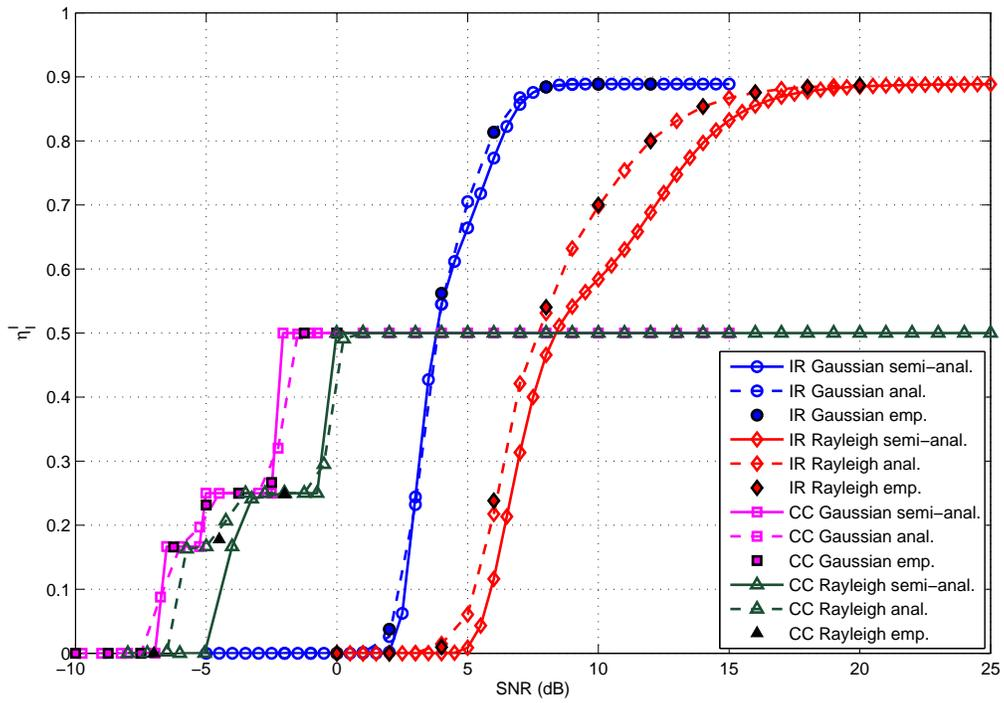
Fig. 3. Efficiency at IP layer for IBS with  $N = 3$ , for CC-HARQ ( $C = 9$ ) and IR-HARQ ( $C = 12$ ).
