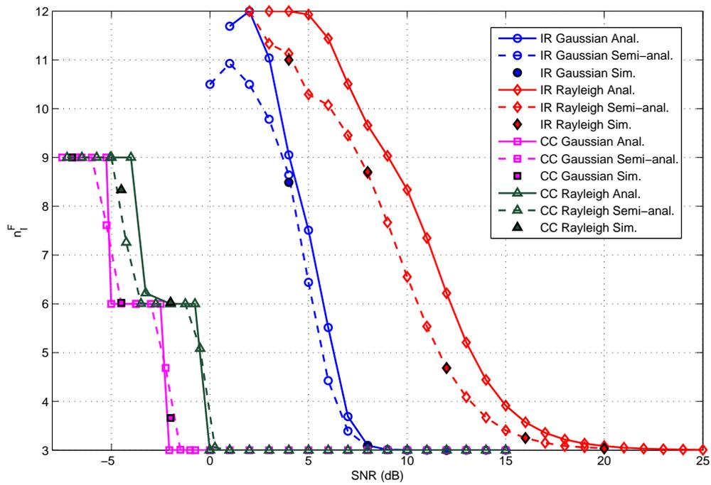
Fig. 5. Delay at IP layer for IBS with  $N = 3$ , for CC-HARQ ( $C = 9$ ) and IR-HARQ ( $C = 12$ ).
