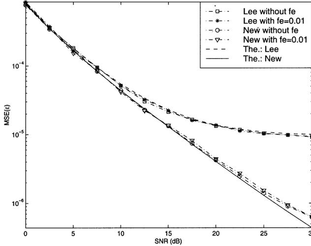
Fig. 4. MSEs of timing delay estimators versus SNR ( $\rho = 0.5$ ).
