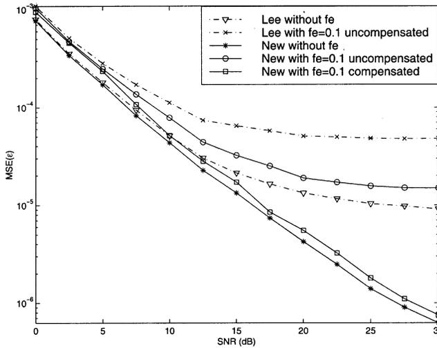
Fig. 5. MSEs of timing delay estimators versus SNR ( $\rho = 0.5$ ).
