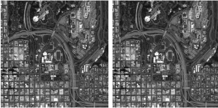
Fig. 10. Green band of the IKONOS image before and after encoding at 0.80 bit/sample.
