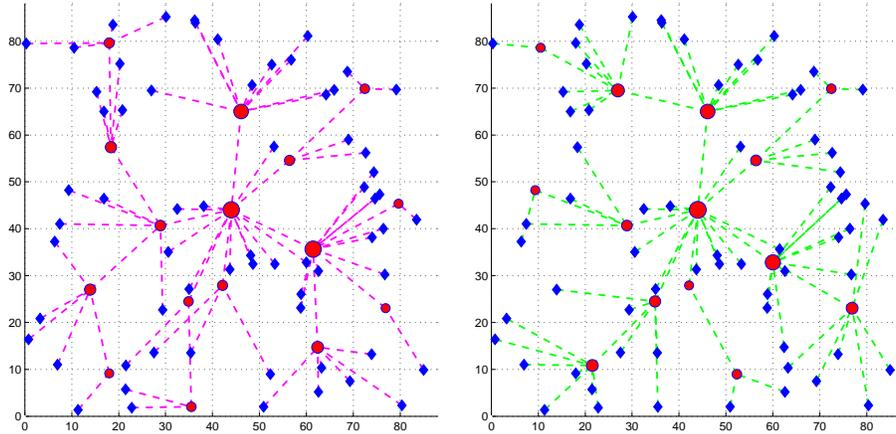
Figure 3. Diffusion trees for 80 nodes in  $88 \times 88 m^2$ , two descriptions. Round spots represent active nodes, the size of the spots is proportional to the number of nodes subscribed.
