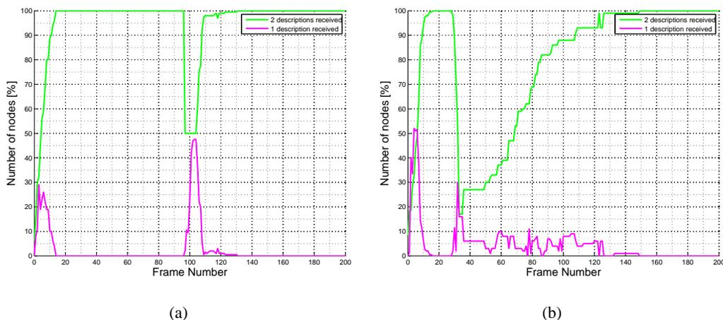
Figure 2. (a) Received frames for 100 nodes in  $140 \times 140 m^2$ ; 100 more nodes connect on the 100-th frame. (b) Received frames for 200 nodes in  $140 \times 140 m^2$ ; 100 nodes disconnect on the 33-rd frame.
