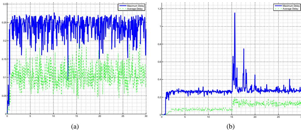
Figure 4. End-to-end delay versus simulation time (both in seconds). (a) Scenario with 60 nodes in  $76 \times 76 m^2$  (compare with figure 1-(a)). (b) Scenario with 100 nodes in  $140 \times 140 m^2$ ; 100 more nodes connect on  $t = 15s$  (compare with figure 2-(a)).
