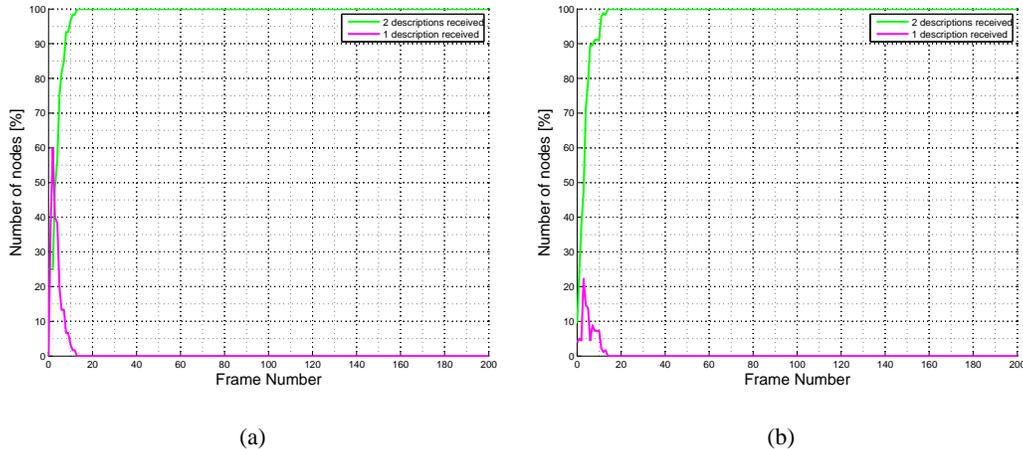
Figure 1. (a) Received frames for 60 nodes in  $76 \times 76 m^2$ . (b) Received frames for 180 nodes in  $132 \times 132 m^2$ .
