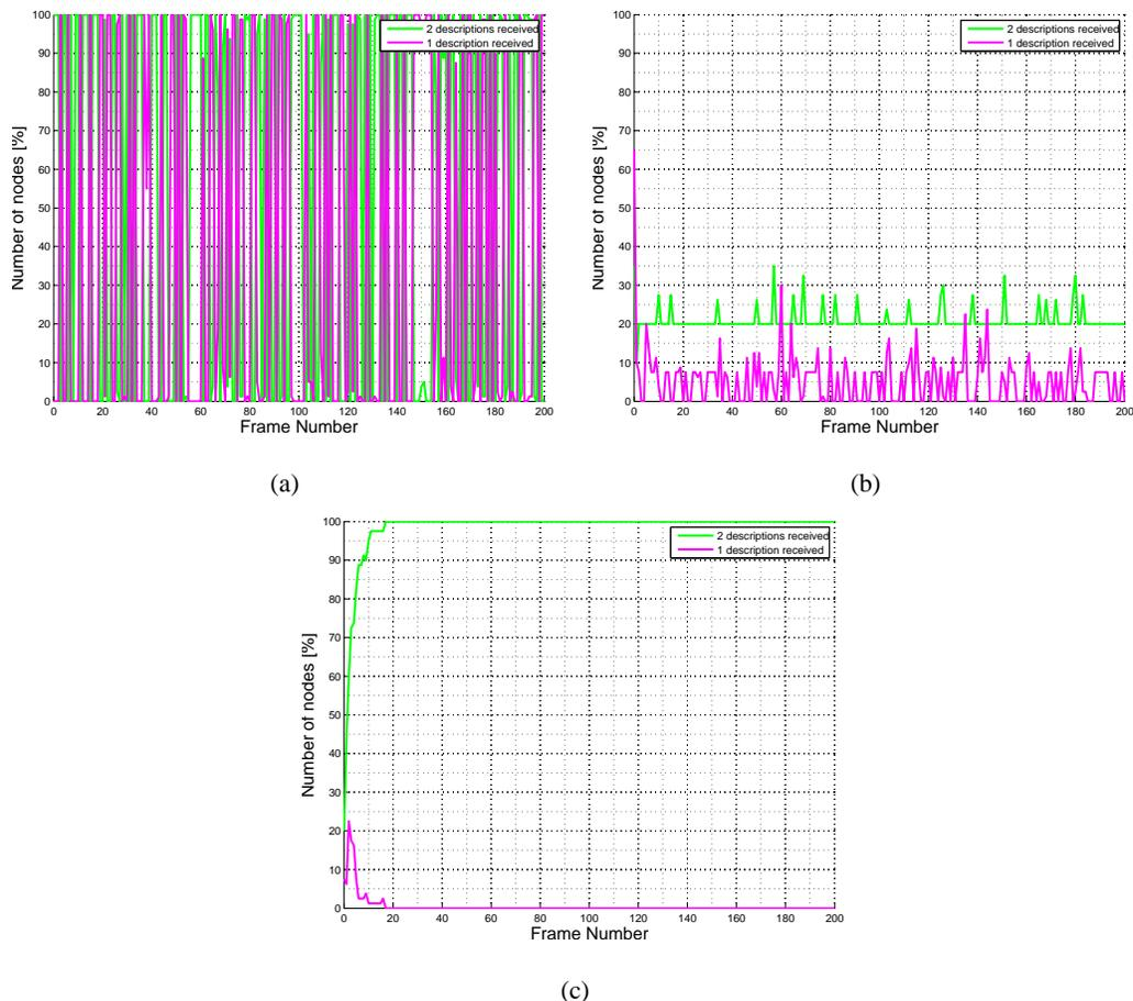
Figure 5. Comparison of delivery rates. (a) Simple Flooding. (b) Probabilistic Flooding with  $p = 20\%$ . (c) ABCD Protocol.
