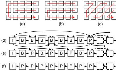
**Fig. 4.** Scan order: (a) spiral, (b) perpendicular, (c) diagonal and Horizontal inter-view reference picture structures: (d) hierarchical, (e) IBP, (f) IPP
