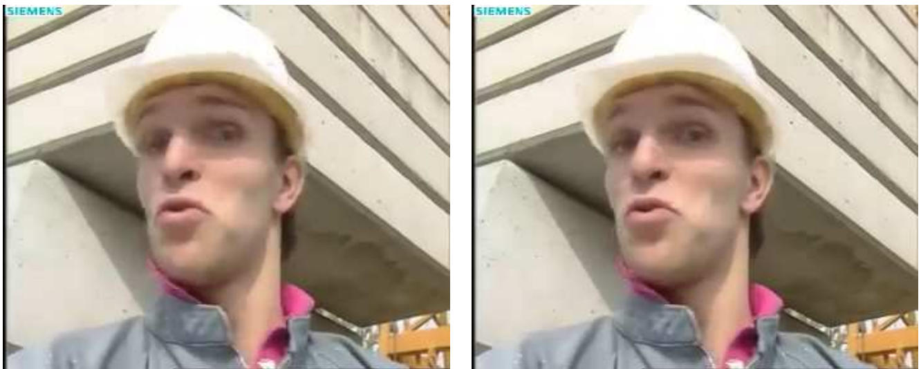
Figure 6. Visual comparison of frame 86 of sequence “Foreman” (CIF sequence, 30 fps, 256 kbps) in reference (left, Y-PSNR=31.67dB) and proposed (right, Y-PSNR=33.55dB) method.
