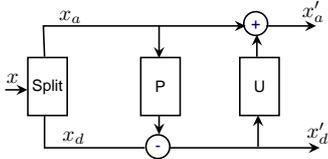
**Fig. 1:** Classical lifting scheme. Analysis.
