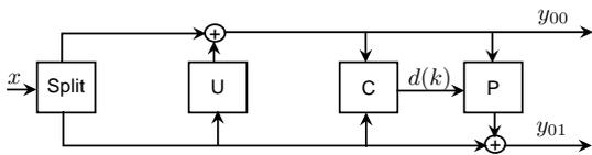
**Fig. 2:** Adaptive prediction lifting scheme
