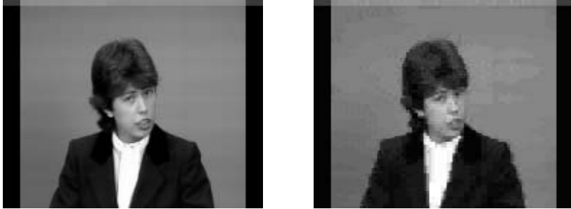
Fig. 5. Sequence CLAIRE: original and encoded frames at 29.3 kbps
