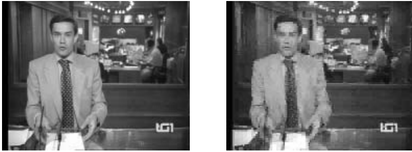
Fig. 4. Sequence NEWS: original and encoded frames at 35.8 kbps
