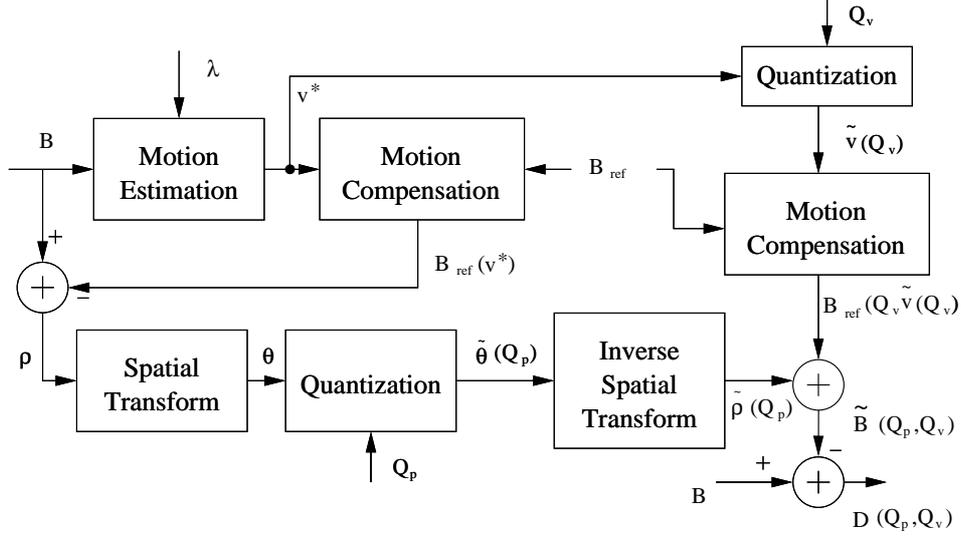
Figure 2. Open loop quantization of motion vectors
