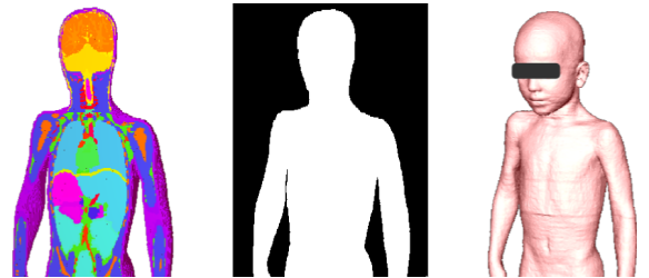
Figure 3: Visualization envelope: Starting from the input voxel grid (left) a binary grid captures the foreground/background interface (middle) from which a surface mesh is sampled for interactive visual feedback (right).
