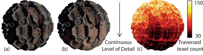
Fig. 5. Continuous geometric LoD: (a) Displaced object rendered at maximum LoD. (b) Our D-BVH is able to render different non-integer LoD for each ray, driven by the screen-space y position of the primary ray. (c) LoD influence on the number of traversed nodes.
