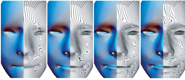
Figure 4: The subdivision of normals can be started from the base mesh or after few levels of geometric subdivision. The images show the results starting with the normals of the base mesh, the normals of the mesh subdivided one time and two times. The right image is shaded with normals computed at the fully subdivided mesh.
