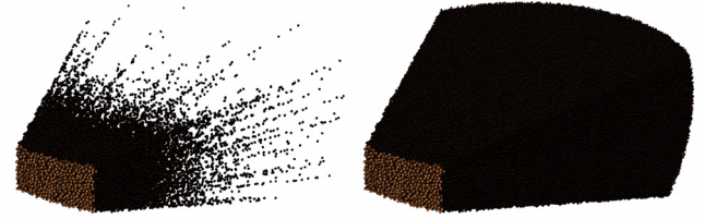
Figure 14: View frustum with (left) and without (right) our grain occlusion culling. Some of the remaining points may actually be hidden, but it is ensured that no visible point is removed.
