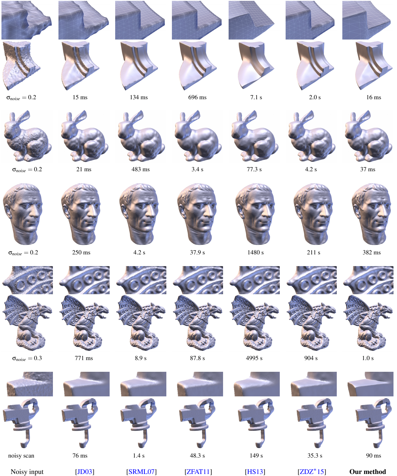
Figure 8: Comparisons for models with synthetic Gaussian noise of standard deviation \sigma_{noise} , and a real noisy scanned model. \sigma_{noise} given in terms of mean edge length.
