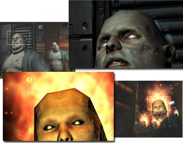
**Figure 2:** As shown in these captures from the game *Doom 3* (id Software), normal mapping and Phong shading provide reasonable shading of the interior of objects, but the piecewise linear shape is clearly visible along contours.
