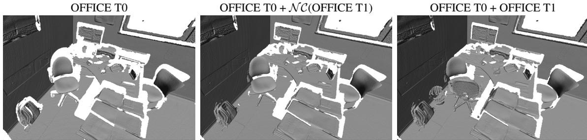
**Figure 16:** Triangulation results from three inputs: (Left) OFFICE T0; (Center) OFFICE T0 plus the no change regions of OFFICE T1; (Right) union of OFFICE T0 and OFFICE T1. The pictures in the center show a more complete reconstruction without inconsistencies due to the intersection of different objects.
