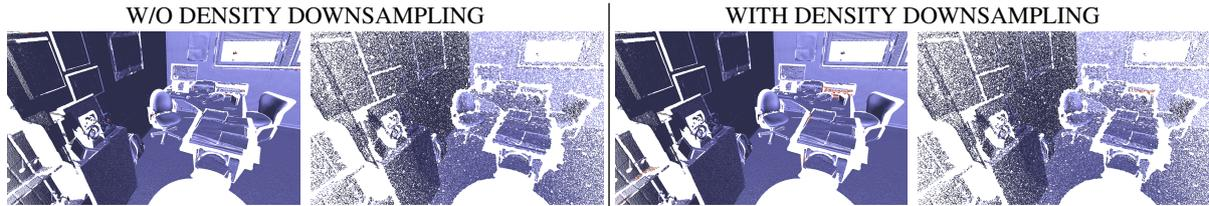
**Figure 13:** Change detection between a scan and its sub-sampled versions to verify the robustness against the point density (OFFICE S1 vs OFFICE S0.125). The left column shows the result obtained using directly the two scans while the right column shows the result with the sub-sampling preprocessing to reduce the scans at the same local density.
