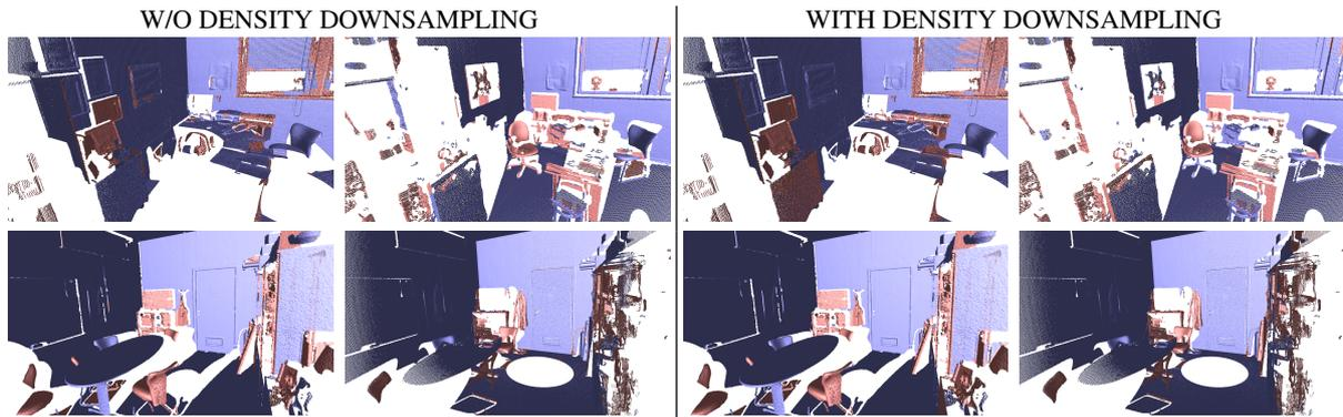
**Figure 14:** Change detection between two scans of the office acquired from the opposite corner of the room (OFFICE P1 and OFFICE P2) and displayed from different viewpoints. The left column shows the result obtained using directly the two scans. The right column shows the result with the sub-sampling preprocessing to reduce the scans at the same local density.
