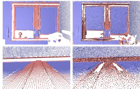
**Figure 15:** Change detection results in noisy point clouds: (Left) OFFICE P1; (Right) OFFICE P2. In this case the detection of change points on the aluminum window frame is due to the high level of noise in the scan OFFICE P2.
