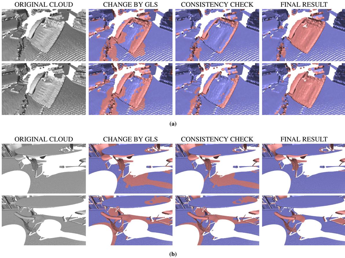
**Figure 7:** Evolution of the change/no-change segmentation (red = change, blue = no-change) during the main steps of the algorithm in the case of critical configurations: (a) a small movement of an object over a plane (a phone slightly rotated over the desk); (b) occlusion (region of the floor occluded by a chair that has been moved before the second scan). For each sub-figure: (Top) OFFICE T0. (Bottom) OFFICE T1.
