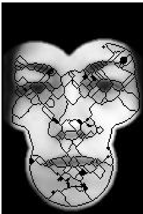
Figure 7.4: Example of an over-segmented image after applying the watershed algorithm.
