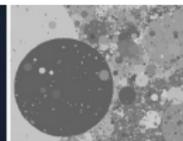
A detail of a target made of a dead leaves pattern, designed to measure Texture Acutance. It is obtained by drawing random shapes that occlude each other in the plane. The dead leaves falling from a tree. The statistics of this model follow the distribution of the same statistics in natural images.
