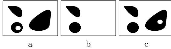
Figure 1: Filtering of a crisp set (a) with a connected operator (b) and with a non-connected operator (c).
