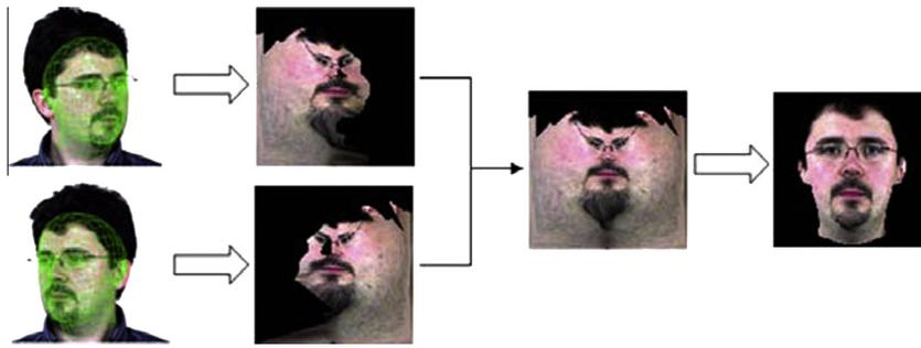
Fig. 6. Pose and shape estimation, texture map extraction, fusion and frontal view generation.
