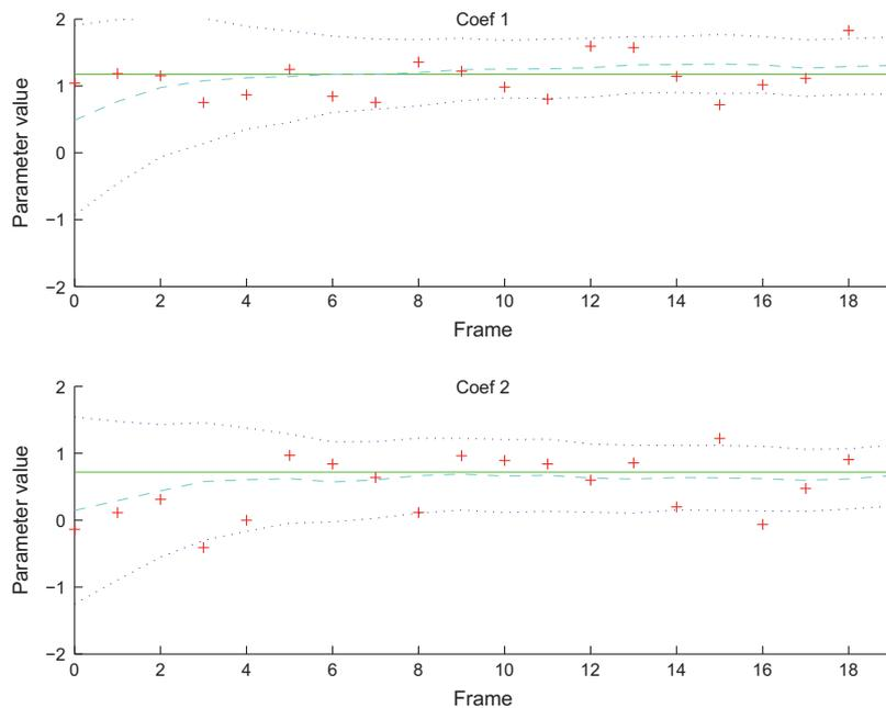
Fig. 13. Evolution of the filter static shape parameters, when the pose is unknown. No noise is added to the input feature points.  $N = 2500$  particles are used, and artificial moves are Gaussian noises with adaptive covariance.
