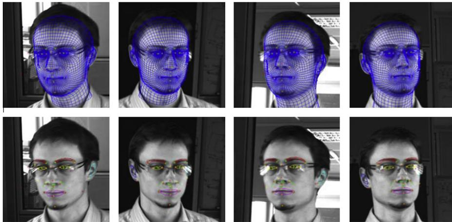
Fig. 18. Projection of the estimated mesh and internal edges on the acquired image at the end of a sequence.
