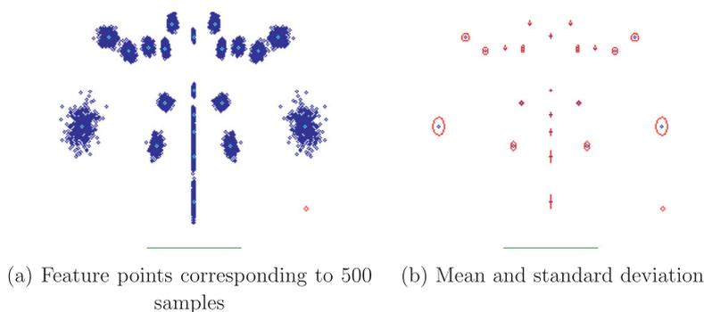
**Fig. 8.** Feature point distribution given the shape model seen frontally. In the right corner at the bottom, a 2 pixel radius circle is represented, corresponding to the standard deviation of the Gaussian noise applied to the positions. The distances between eyes on these two images are around 80 pixels, which is represented by the green line on the bottom. (For interpretation of the references to color in this figure legend, the reader is referred to the web version of this article.)
