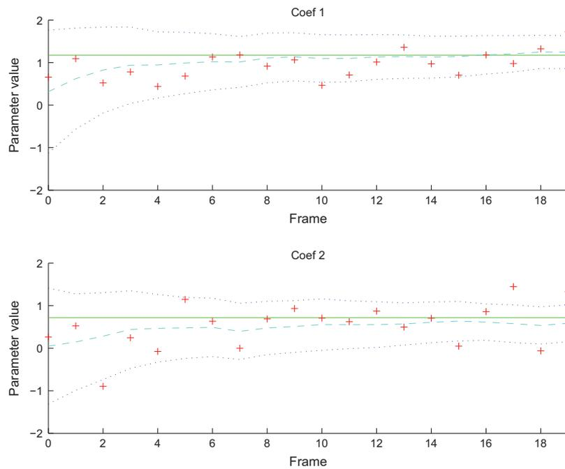
**Fig. 14.** Evolution of the filter static shape parameters when the pose is unknown. A Gaussian noise ( $\sigma = 2$  pixels) is added to the input feature points.  $N = 2500$  particles are used, and artificial moves are Gaussian noises with adaptive covariance.
