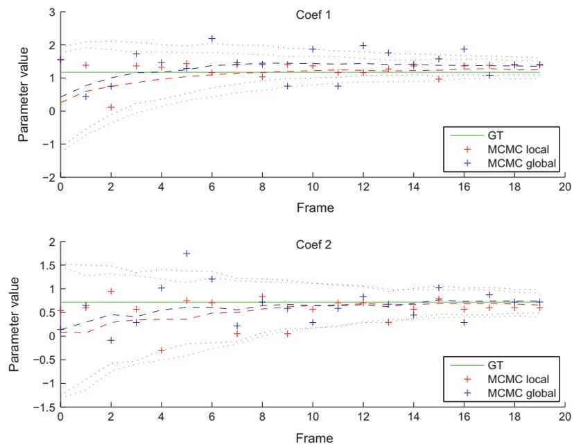
**Fig. 15.** Evolution of the filter static shape parameters when the pose is unknown.  $N = 2500$  particles and MCMC moves are employed.
