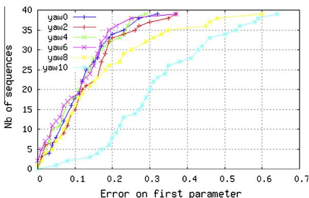
**Fig. 10.** Robustness of the first shape parameter estimation depending on the initial yaw angle error, varying from 0 (yaw0) to 10 degrees (yaw10). The Y-axis indicates the cumulative number of sequences for which the error on the first parameter is below a threshold (read on the X-axis).
