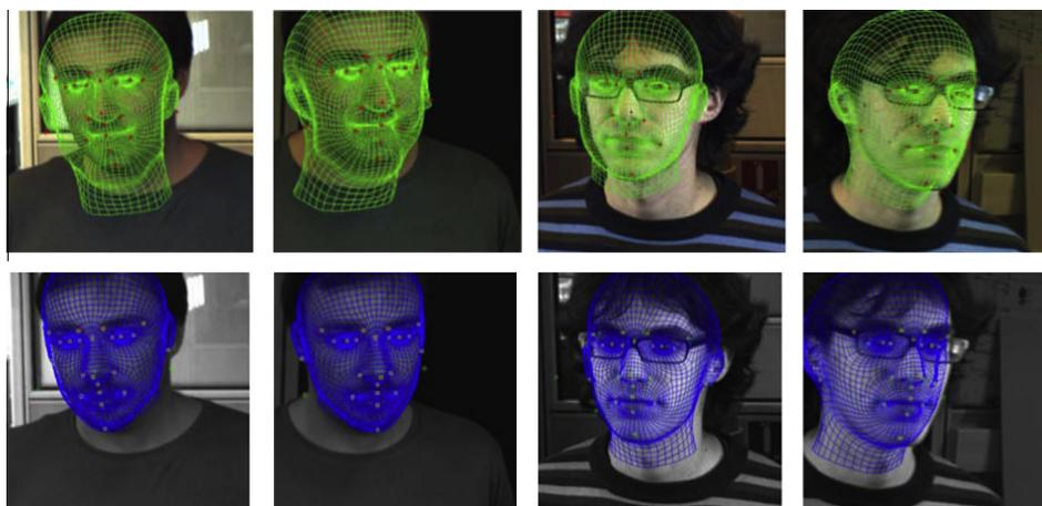
Fig. 20. Comparison between the pose and shape estimation computed by Levenberg–Marquardt (in green) and the one computed by particle filtering (in blue). (For interpretation of the references to color in this figure legend, the reader is referred to the web version of this article.)
