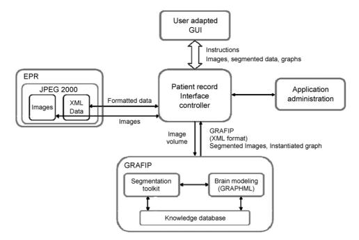
Fig. 1. Functional scheme of the proposed EPR application.
