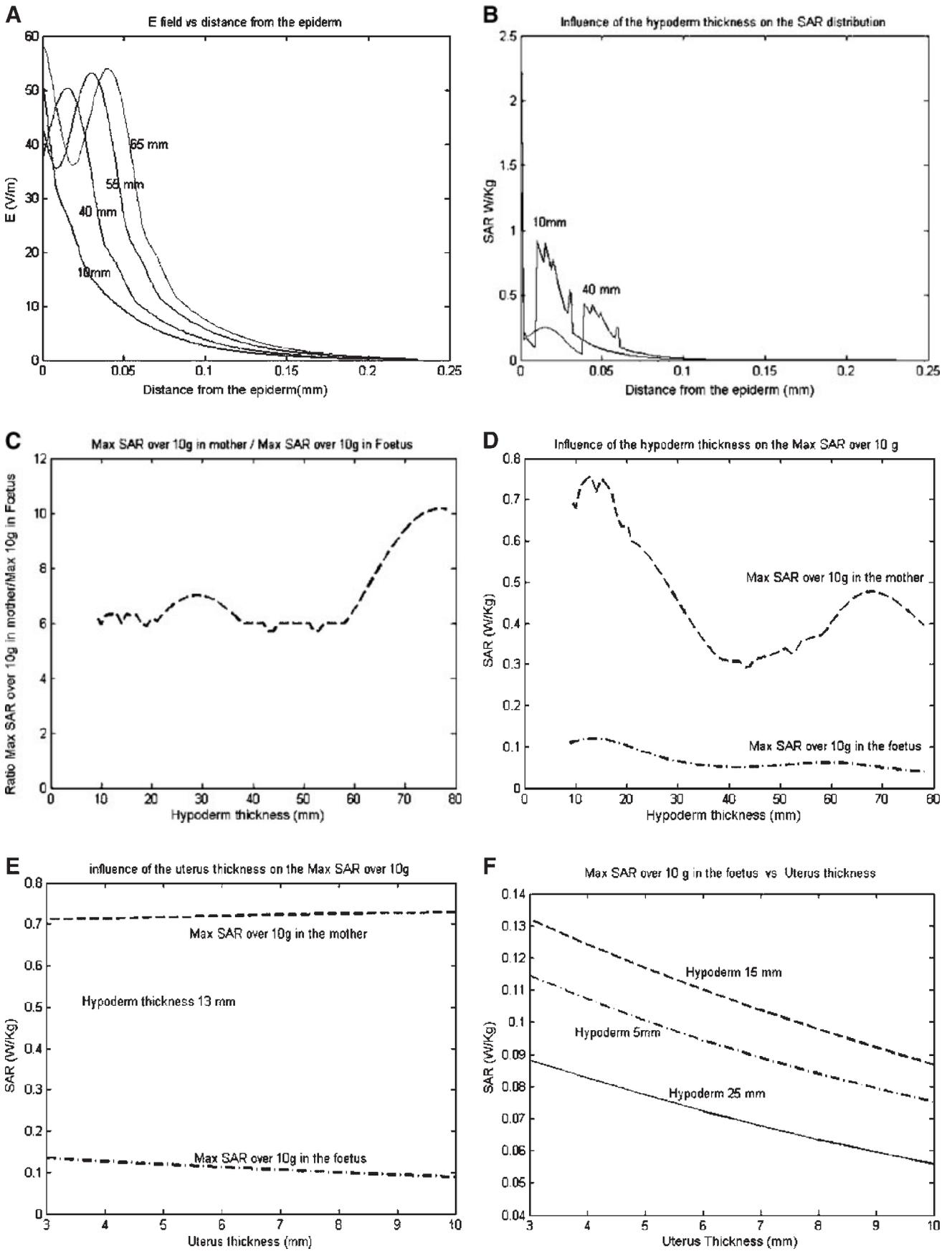
Fig. 20. E field (A) and SAR (B-F) assessment in foetus using a multilayer approach at 900 MHz.
