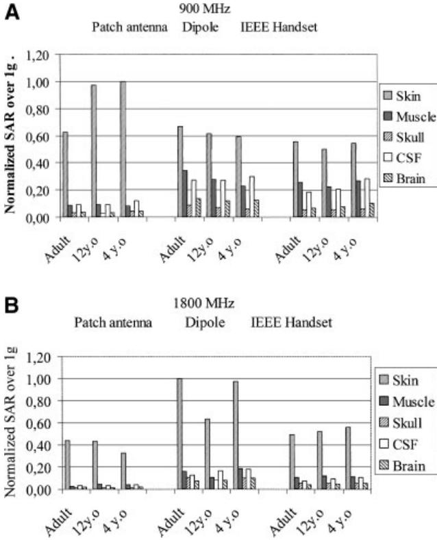
Fig. 13. **A:** Normalized (to 250 mW) SAR over 1g induced in different tissues of adult and child like heads versus handset at 900 MHz. **B:** Normalized (to 125 mW) SAR over 1g induced in different tissues of adult and child-like heads versus handset at 1,800 MHz.
