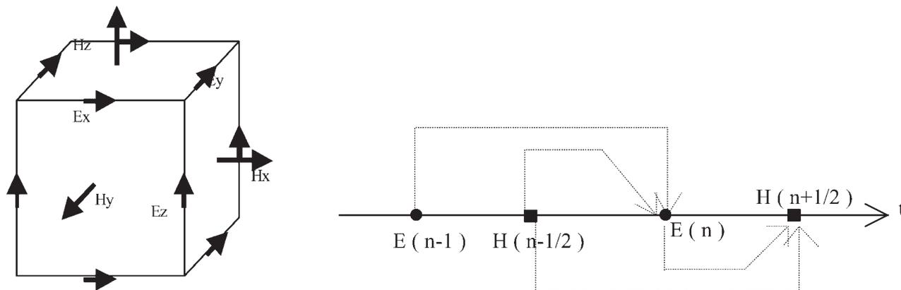
Fig. 1. Yee cell and the "leap frog" scheme of the FDTD method.
