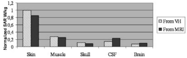
Fig. 15. Normalized SAR (to the max SAR over 1 g in the head skin derived from visible human) for different tissues in a 12 year old child head (child like derived from the visible human and model from MRI).
