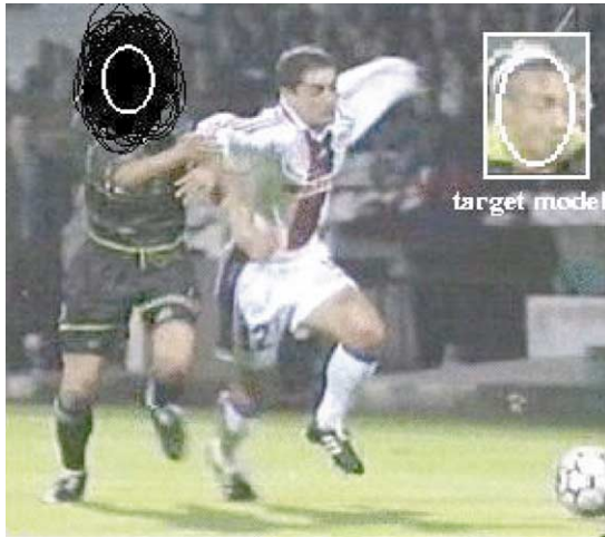
Fig. 1. A color-based target model and the different hypotheses (black ellipses) calculated with the particle filter. The white ellipse on the left represents the expected object location.
