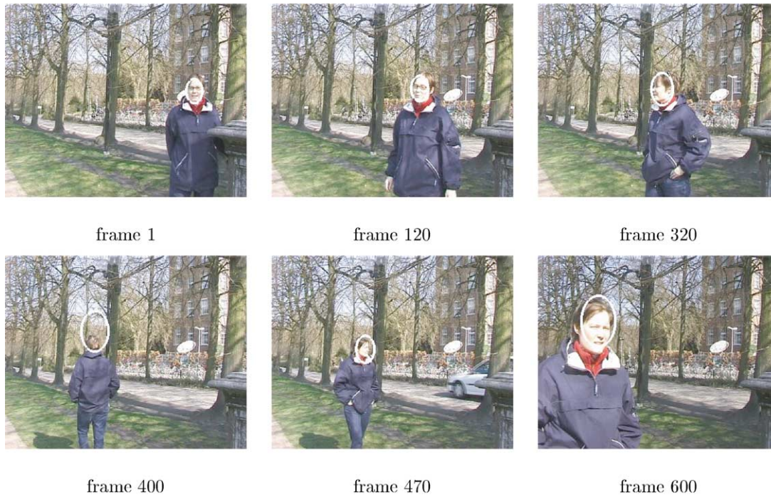
Fig. 16. The face sequence shows the tracking performance with an adaptive model. The tracker handles a large object motion and illumination changes using N = 100 samples.
