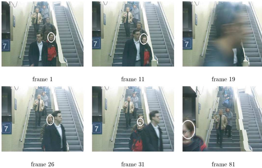
Fig. 14. The moving stairs sequence shows the robustness of the color-based particle filter against occlusion and strong scale changes. Furthermore, in frame 26 the effect of the initialization is illustrated.
