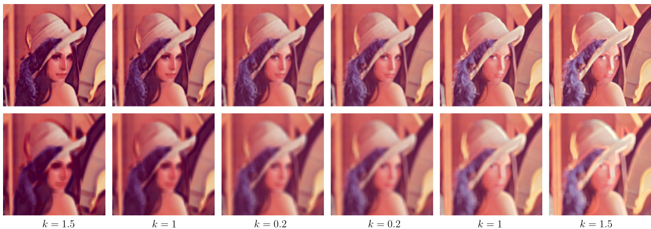
Fig. 11. Pseudo-erosions (left half) and pseudo-dilations (right half), PPM, SE size is 5 \times 5 (top row) and 11 \times 11 (bottom row). (For interpretation of the references to color in this figure caption, the reader is referred to the web version of this article.)
