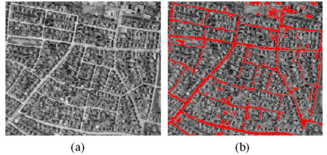
Fig. 12. Second test results. (a) VHR IKONOS example containing 300 \times 300 pixels; and (b) road map result.
