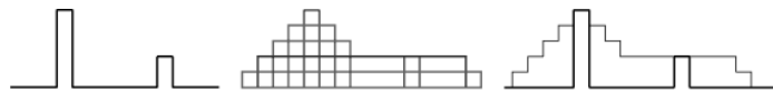
Figure 16. Effect of the viscous dilations on walls of different altitudes (case of a oil type of fluid).
