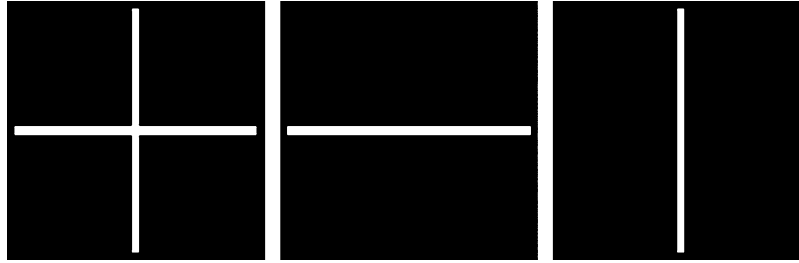
Fig. 1. Overlap in perceptual grouping: the cross (left) is perceived as two bars, one horizontal (middle) one vertical (right). The centre pixel belongs to both perceptual groups.
