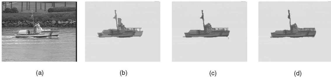
Fig. 15. COASTGUARD sequence: (a) one input image, (b) edge-based segmentation, (c) graph cuts, and (d) tensor voting.
