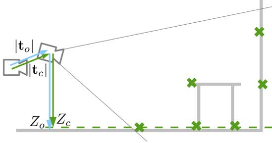
Figure 3: The ground plane is correctly identified by the 4<sup>th</sup> step of sparse 3D reconstruction. The camera's height  $Z_c$  above it may safely be assumed to equal the altitude  $Z_o$  measured by the on-board ultrasonic sensor.
