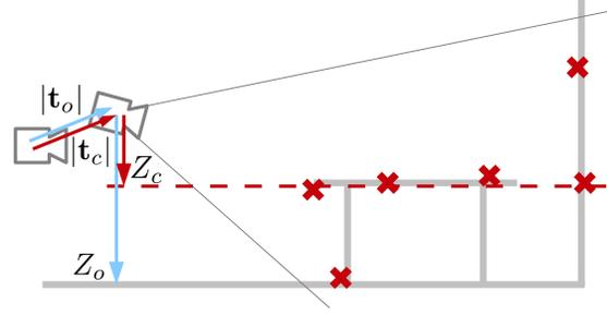
Figure 4: The tabletop is mistaken for the ground plane. The 3D points' distances and the camera's motion  $\mathbf{t}_c$  are over-estimated by a common factor, which can be corrected by incorporating  $\mathbf{t}_o$  from on-board odometry.
