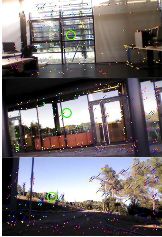
Figure 6: Imperfect sparse 3D reconstructions: A path through a window is planned because of too few correspondences on its blinds (top). Mostly mirrored points are reconstructed (middle). Difficult lighting caused erroneous estimates of camera motion and 3D point distances (bottom).
