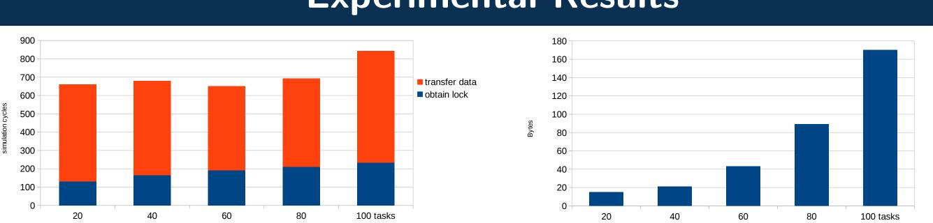
► Latency (left) and buffer fill state (right). Clustered platform, 8 MIPS32 processors, 6 classification and 2 scheduling tasks
