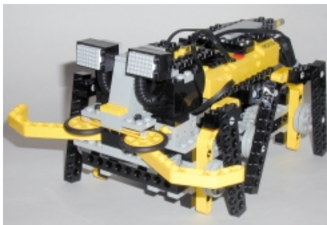
Six-legged pet built by Jin Sato includes a home-built light-emitting diode array for displaying different eye expressions.
