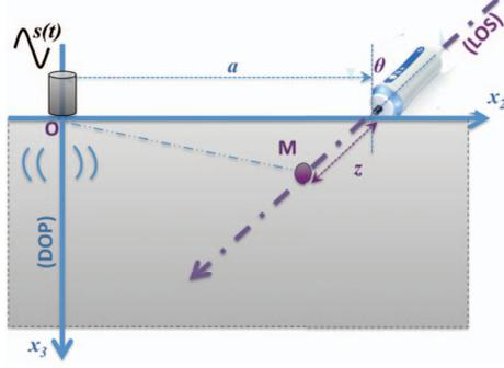
**Fig. 1.** Setup of transient elastography scanning. Parameters include the direction of propagation (DOP) of the shear wave and the line of sight (LOS) used to record the RF lines. In the general case, the LOS can be shifted (by  $a$ ) and tilted (by angle  $\theta$ ) with respect to the DOP.
