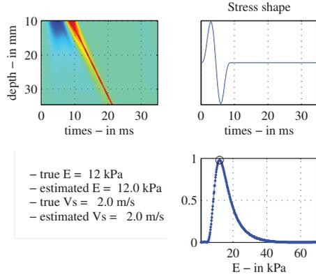
**Fig. 2.** ML estimation of  $E$  on simulated data. (top left) Simulated displacement field. (top right) Stress temporal profile in arbitrary unit (A.U.) applied with a cylindrical piston. (bottom right) Likelihood criterion in A.U. versus  $E$ .
