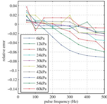
**Fig. 3.** Relative errors of ML elasticity estimations versus stress frequency using FEM simulations with different  $E$  values.
