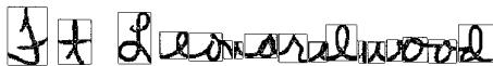
Fig. 15. Oversegmenting. Note that letters that contain valleys have been dissected into multiple parts. However, no merged characters remain, so that a correct segmentation can be produced by recombination of some of the segments.
