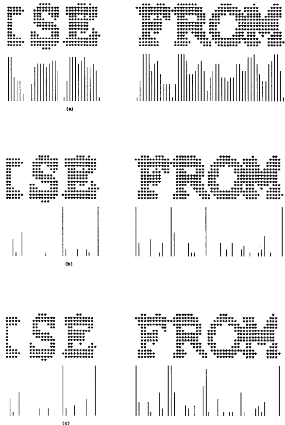
Fig. 6. Dissection based on projection: (a) Vertical projection of an image. It is an easy matter to detect white columns between characters, and regions of light contact. The function fails, however, to make clear the O-M separation. (b) Differencing measure for column splitting. The function from [1] is based on a second difference of the projection. This gives a clear peak at most separation columns, but may still fail for the O-M case. (c) Differencing measure after column ANDing. The image transformed by an AND of adjacent columns, with the difference function of (b) applied to the transformed image. The AND operation tends to increase separation, leading to a better defined peak at the O-M boundary.
