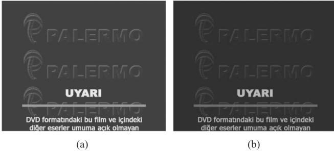
Fig. 5. Comparison results of histogram smoothing and weighted histogram approximation for image Palermo . (a) Histogram smoothing using (9) with \gamma = 1000 and \lambda = 1 , (b) weighted approximation using (12) with \lambda = 1000 .
