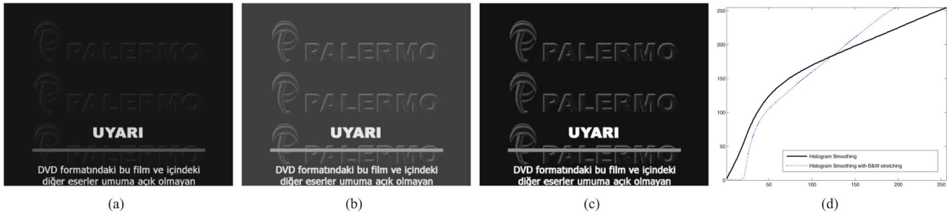
Fig. 7. Comparison results of histogram smoothing with and without B&W stretching for image Palermo . (a) Original image, (b) enhanced image using (9) with \gamma = 1000 and \lambda = 1 , (c) enhanced image using (14) with \gamma = 100 , \lambda = 1 , and \alpha = 5 , (d) mappings for the two enhanced images in (b) and (c).
