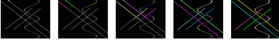
FIGURE 4.6: Evolution of clustering algorithm for a synthetic example. The coloured pixels belong to clusters, whereas the grey pixels have not been processed yet. Each colour represents a single cluster. In this simple situation, each final cluster represents a trajectory.
