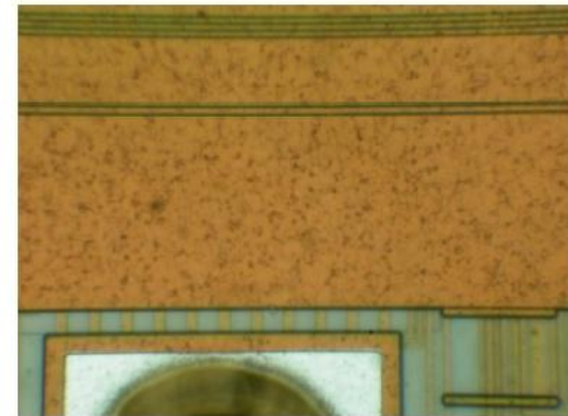
Top metal layer on microchip PIC16F877A microcontroller
