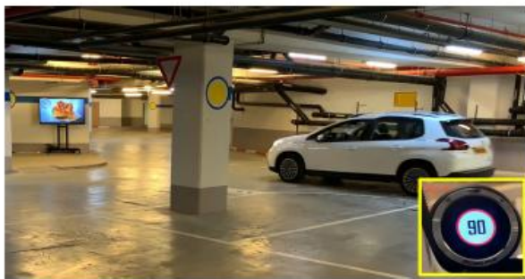
Figure 5: Mobileye issues an alert about a phantom road sign after the phantom speed limit was detected in the upper left corner of the digital billboard.
