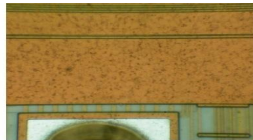
Top metal layer on microchip PIC16F877A microcontroller
