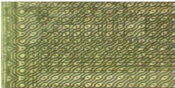
Top metal sensor on ST16 smartcard
