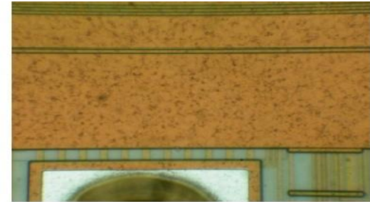
Top metal layer on microchip PIC16F877A microcontroller
