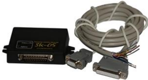
Figure 2.4: DPF emulator for Toyota, source dpf-toyota.com
